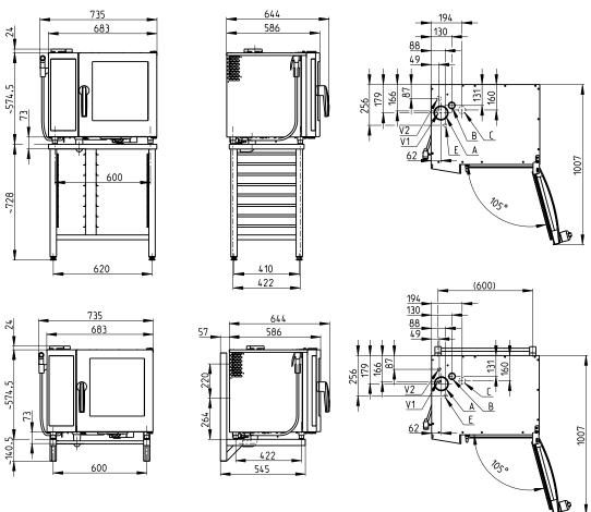
A - Flap valve, B - Chimney, C - Drain, E - Electricity, V1 – Untreated water, V2 – Treated water
