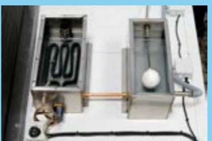
Steam generator's functioning does not affect chamber's temperature: increases proofing homogeneity.
